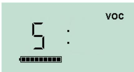
Press the multi-function button to initiate the Span stage. The screen will display an 'S'.
