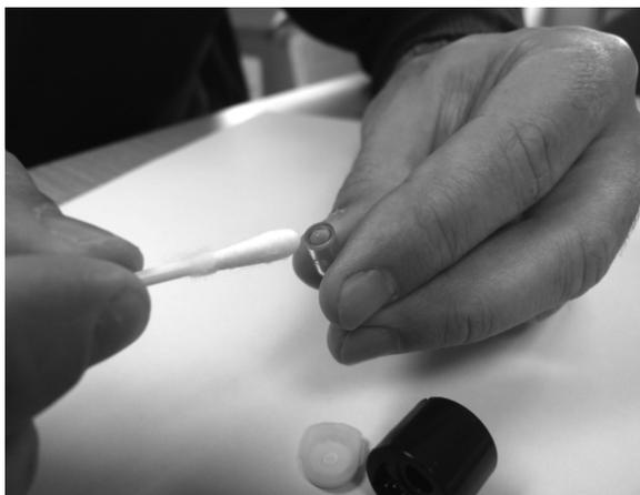
3. Continue polishing until an audible “squeaking” is made by the cotton bud with compound moving over the window surface (usually within fifteen seconds).
