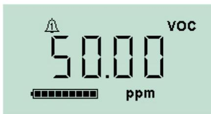
If the detected gas level triggers a low-level alarm, the display screen will flash orange, and the lights on the top of the unit will flash red.
