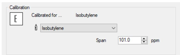
From the drop-down list, select the gas that the Cub is calibrated for.
