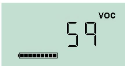
The screen will change and display a live reading from the sensor. *This number does not relate to gas concentration, it simply indicates if the sensor output is changing.*
