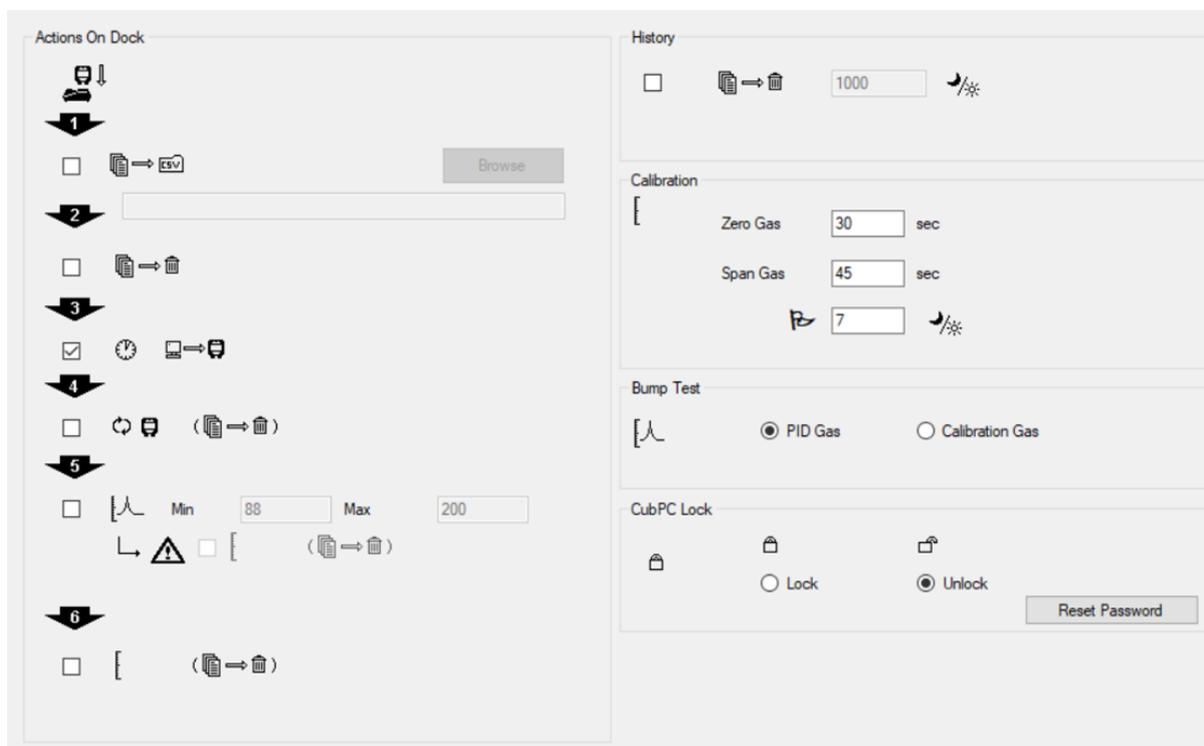
This page is used to set preferences for the CubPC software, such as actions taken when Cubs are docked.
