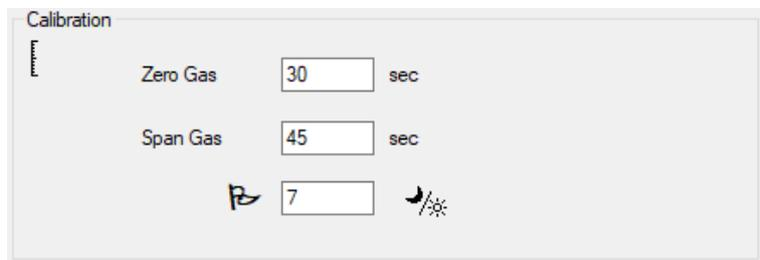
In both the **Zero Gas** and **Span Gas** fields enter the number of seconds that the Zero Gas and Span Gas are to be sent to a connected Cub when it is being calibrated.
