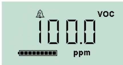
If the detected gas level triggers a high-level alarm, the display screen and the lights on the top of the unit will flash red.
