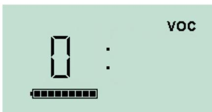
This initiates the Zero stage of the procedure. The screen will display a '0'.
