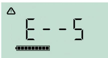
If there is no significant difference between the Zero and Span levels the calibration will be invalid and E- - 5 will be displayed. If this occurs, the previous valid calibration levels will be used.
