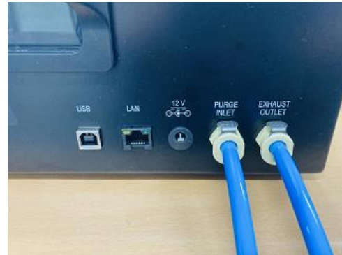
Exhaust Outlet - 1/8" Tube connect to ventilation
