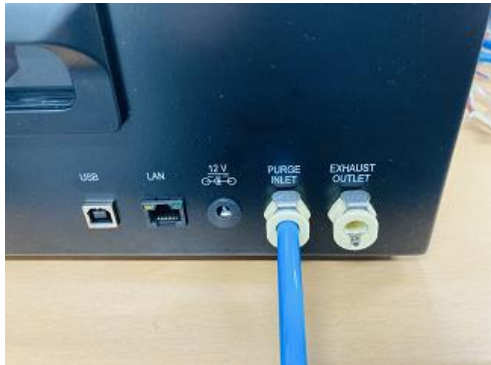
Purge Inlet - 1/8" Tube connect to Clean Air
