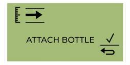
Attach the bottle before you start calibration. This ensures that benzene is flowing through the benzene monitor system before the start of the calibration.
