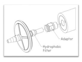
Ensure the external hydrophobic filter and any exhaust or inlet probe lines are connected. Switch on or connect the power supply.
