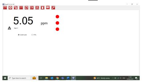
This tab displays in real time what is displayed on the benzene monitor screen. A radio button allows the user to switch between the current cycle reading and the calculated STEL.
