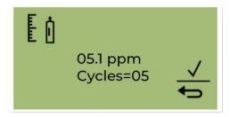
Move the cursor to the ppm value. Use Switch 2 to cycle through the values to the benzene concentration of the bottle.
