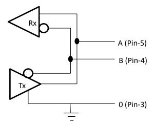
To connect a 120R termination resistor across 'A' and 'B': connect a jumper on L1 between the middle pin and 120R pin. (Refer to Note 1 of <u>Terminal Block-2</u>, Installation).
