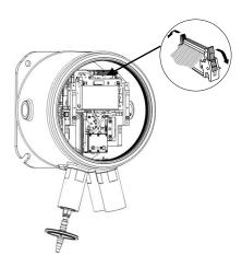
Press the 'wings' down to release the ribbon cable at the top of the Detection Module.
