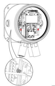
If the module is in its correct position, the screws will engage in the threads and turn freely.
