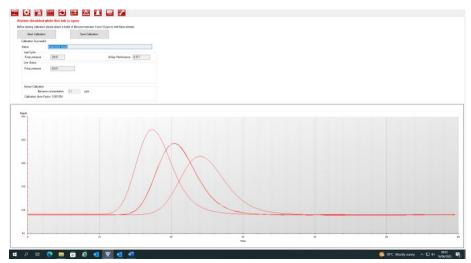
Attach a bottle between 0.1 ppm – 20 ppm Benzene to the inlet flame-arrestor before you start calibration. This ensures the benzene is flowing through the benzene monitor system before the start of the calibration.
