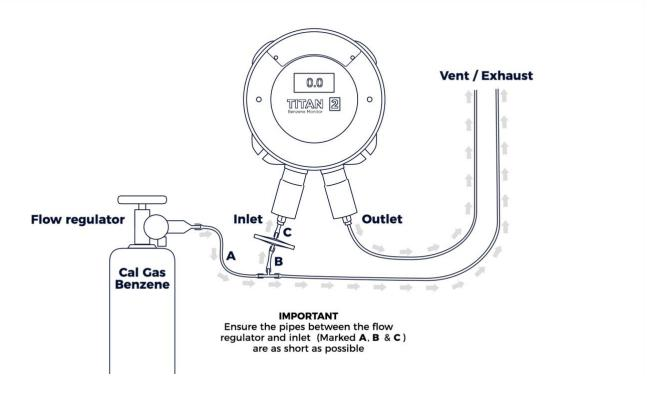
If the benzene monitor does not display the gas concentration given by the bottle, calibrate the benzene monitor to give the correct readings. Refer to:
