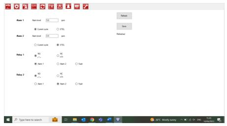
You can set each alarm to operate when the STEL or Current level of Benzene reaches a set value in ppm.
