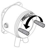
Turn counter-clockwise to unscrew the front cover.
