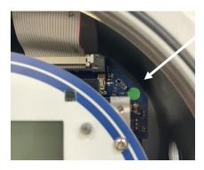
Connect a PC to the USB or RS485 connection and use benzene monitor PC software to set the date and time. Refer to <u>Settings</u>.
