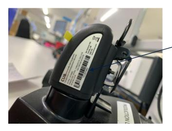
The Serial Number is located underneath the barcode. TC – 6 numbers (TC-XXXXXX)
