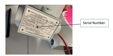
Whether this label is on the side or the back of the instrument, it will still look the same and the Serial Number is located in the same area on the label.
